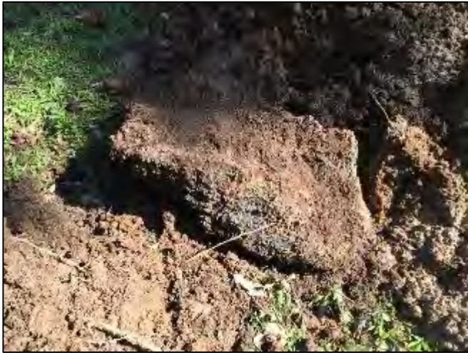
Plate 7 – Asphalt used as fill in the former dam.
