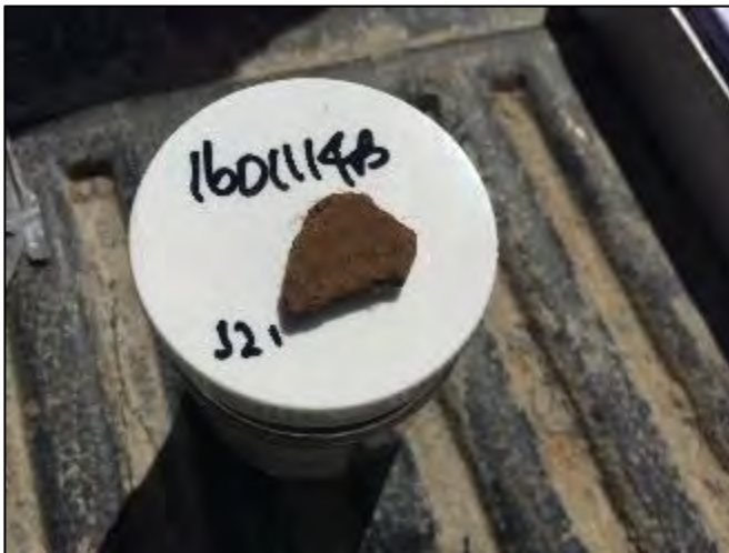
Plate 33 – Fragment of ACM identified in reworked topsoil at S21.
