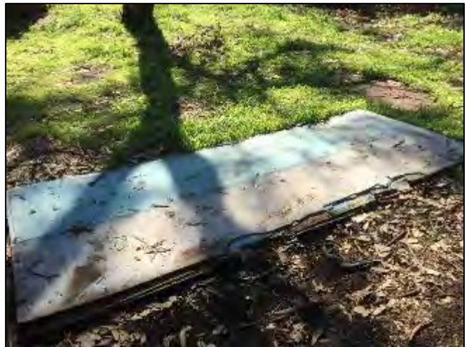
Plate 18 – Sheets of fibre cement sheeting. Did not appear to be ACM.
